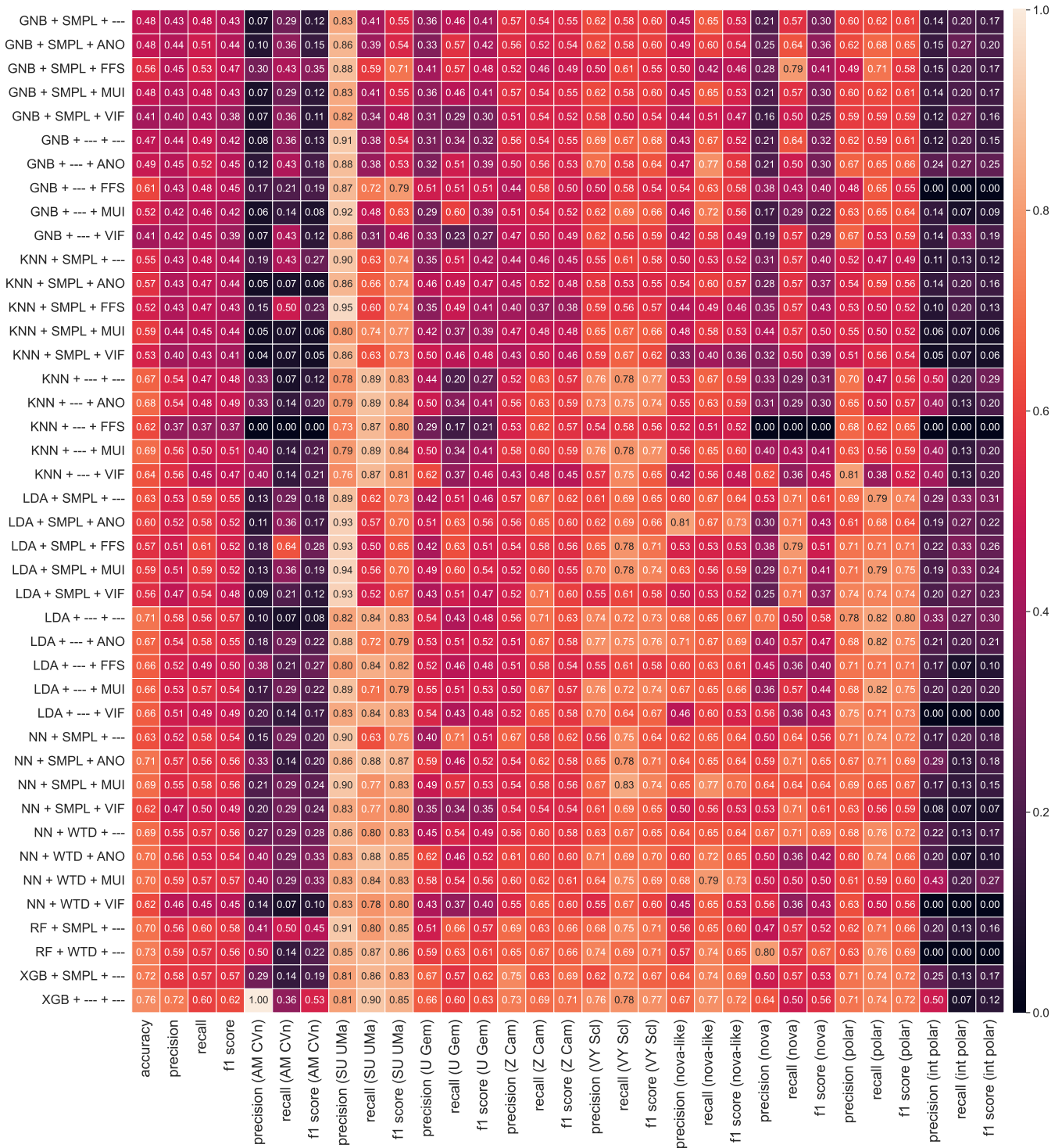
Figure 3. Presented as a heatmap, the accuracy, and the macro average quantities of precision, recall, and F1-score for each classifier variant. Alongside these are the precision, recall, and F1-score for each class. Classifiers are labelled as follows: classifier + class balancing method + feature selection method. Classifier abbreviations are as described in the text, the class balancing methods are abbreviated as SMPL, WTD, or —, depending on whether over/under sampling methods, class weighting, or no class balancing method was implemented, respectively. Feature selection methods are abbreviated as ANO, FFS, MUI, VIF, or —, for one-way ANOVA, forward feature selection, mutual information, variance inflation factor, or no such implementation (full set of features used), respectively.
